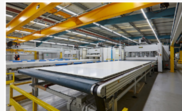
'SMART' GRP sidewall during the production process.
